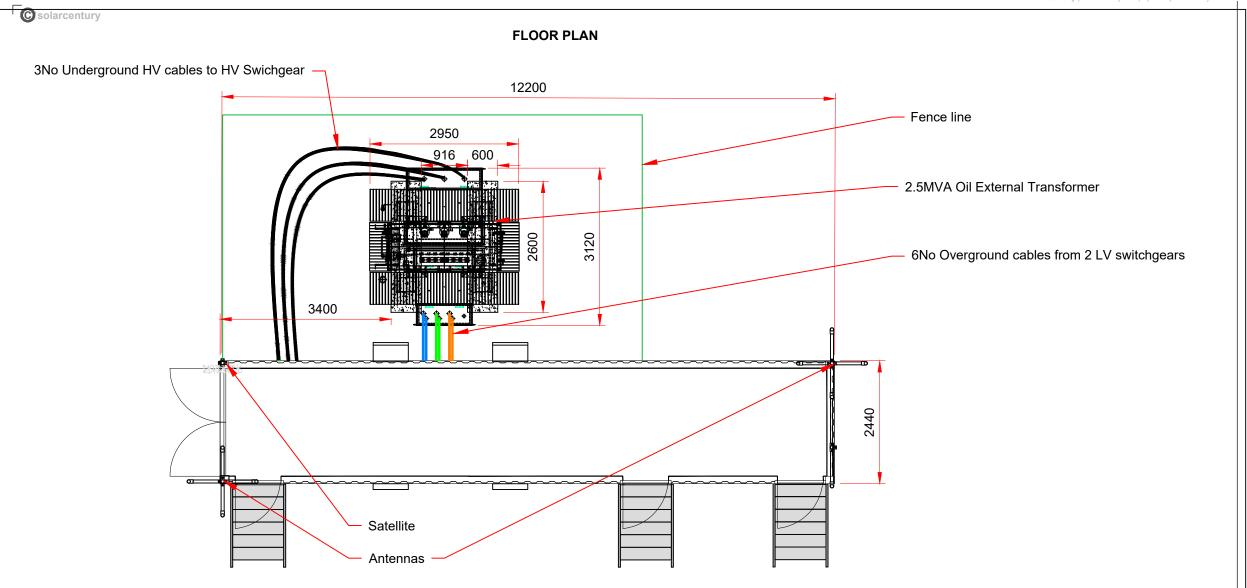
Modified steel shipping container consisting HV & LV Switchgear, comms equipment and storage space
